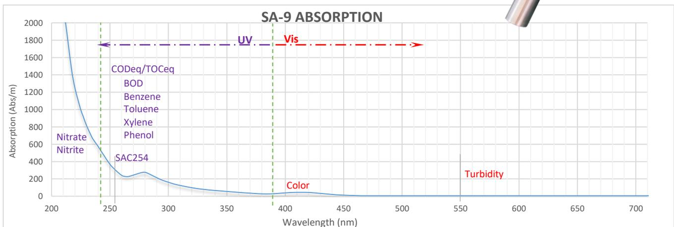
The validated spectral calibration by SA-9 uses multiple wavelengths to monitor and compensate each sum parameter,
